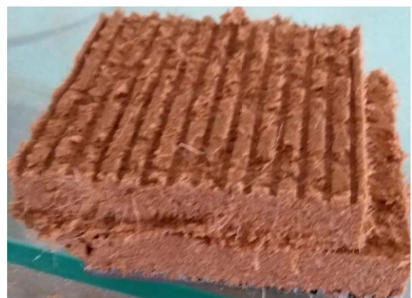
Fig. 3: A typical view of reinforced sand specimen after shearing
